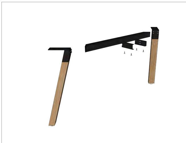
STEP 1: Assemble 2x end leg frames to the legs. Total 6 x M6 bolts per leg.
