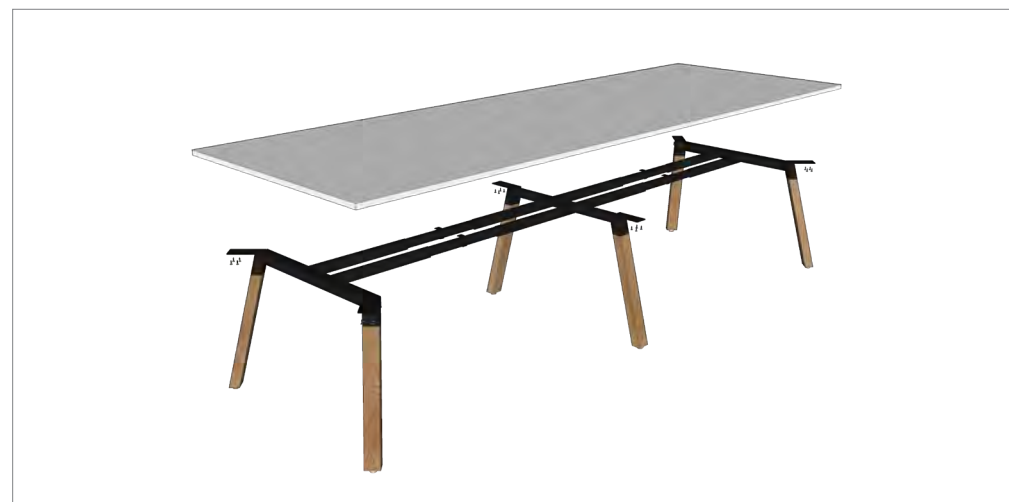
STEP 5: Fix worktop to frame using 4 x ST8 – 23 mm screw per leg, 1 x 23mm screw per rail.
